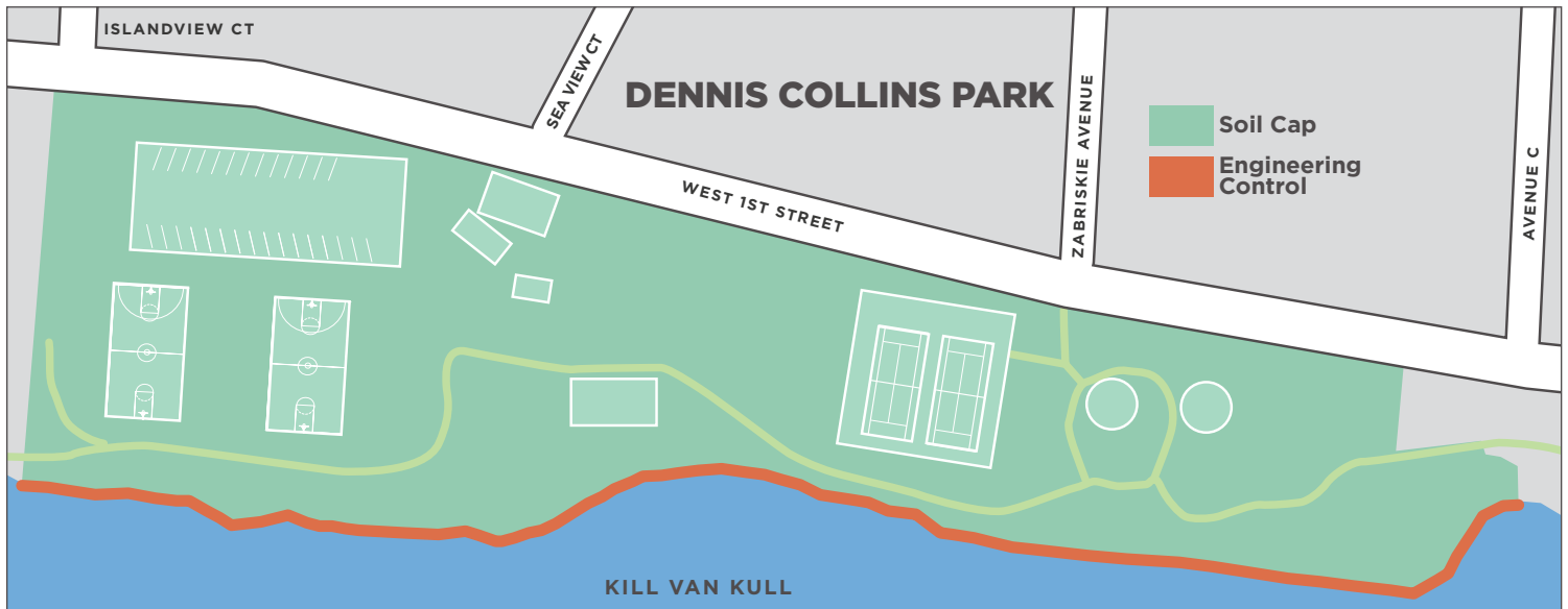
PPG wants to install a 2-foot layer of soil on roughly 9 acres of the park and a new revetment on the adjacent shoreline.
